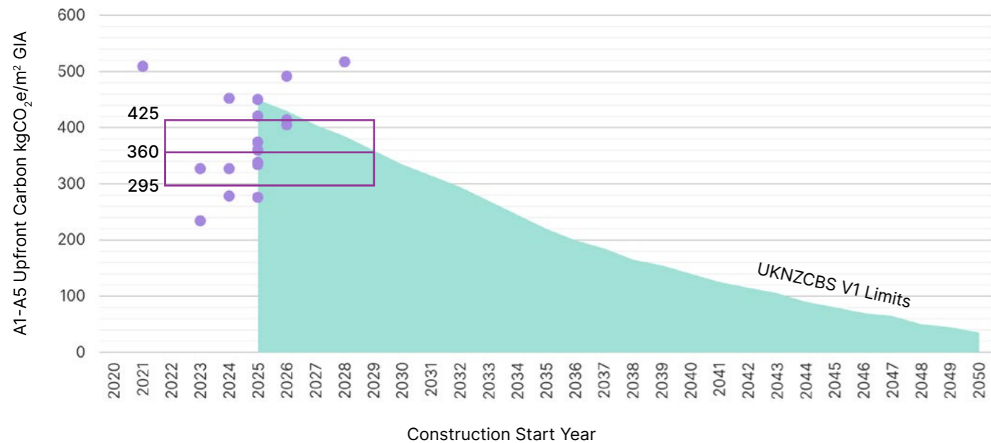
Retrofit Shell & Core + Cat A: A1-A5 Upfront Carbon for London Office Buildings
