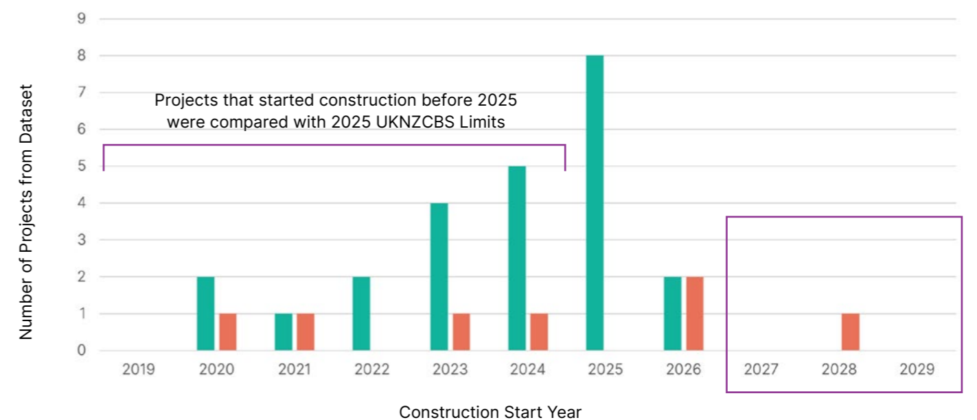
Number of Retrofit Projects Passing/Failing any of the three UKNZCBS limits (S&C, S&C+Cat A or Whole Building)
